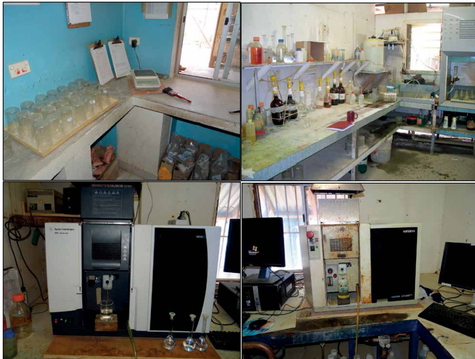
Figure 4.20 Photographs of Tolukuma mine laboratory weighing, wet chemistry digest areas and AAS equipment
